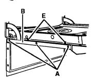
Pull lower edge of panel assembly out and down.
